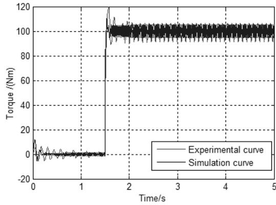
Fig. 4. Response of motor torque output
