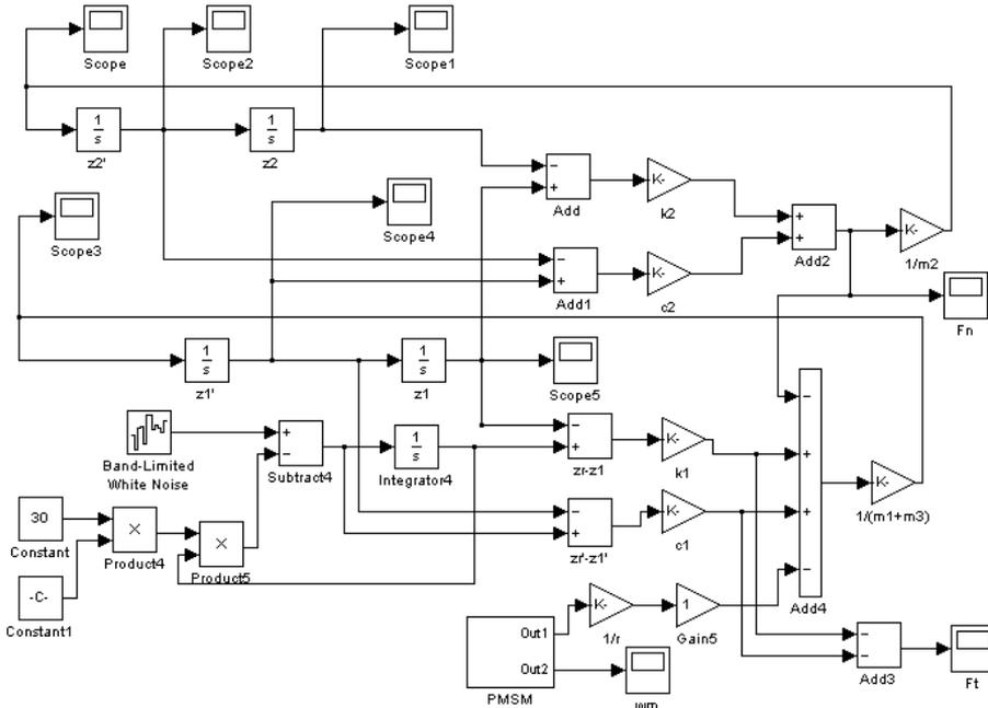
Fig. 8. The vertical vibration Simulink model of 1/4 vehicle
