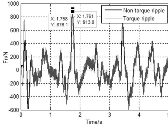
Fig. 9. Response of the vibration input  $F_n$  of sprung mass  $m_2$
