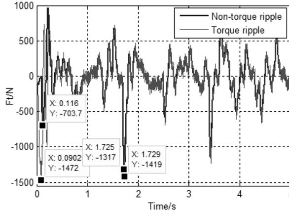
Fig. 10. Response of the dynamic load  $F_t$  of wheel
