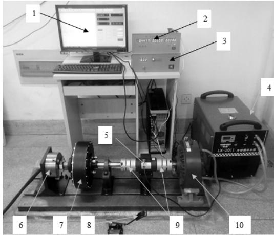
Fig. 7. Motor test bench. 1- PC; 2- Rotational speed & torque collecting instrument; 3- Load controller; 4- Circulating cooling water tank; 5- Motor speed & torque sensor; 6- Three jaw chuck; 7- Permanent magnet synchronous motor; 8- Motor speed control pedal; 9- Double diaphragm coupling; 10- Magnetic powder brake.
