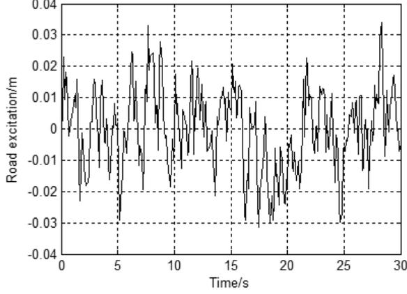
Fig. 2. The curve of Class-B Road excitation electric vehicle (speed of vehicle: 30 m/s)
