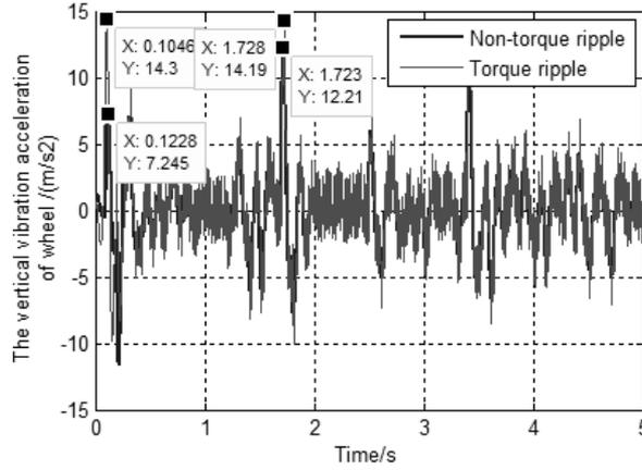
Fig. 11. Response of the vertical vibration acceleration  $\dot{z}_1$  of wheel
