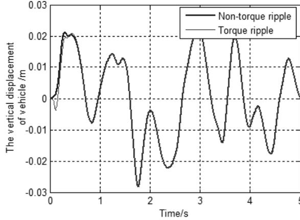
Fig. 16. Response of the vertical displacement  $z_2$  of vehicle
