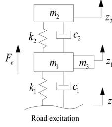
Fig. 1. 1/4 vehicle vertical vibration model of in-wheel-motor
